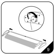
9. If there isn't sufficient tension to fully retract the banner, insert the supplied tool into the hole shown and turn clockwise until the banner is full retracted, then turn an additional 4 to 5 revolutions
