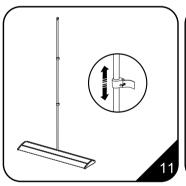
11. Open the lever locks and extend the pole to the desired height and close the levers to lock the pole in that position. Alternately, you can follow steps 12 and 13 and fix the head rail to the pole before extending it.
