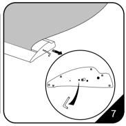
7. Remove the magnetic end caps from the base. While holding the graphic securely, remove the Allen key to release the spring tension
