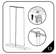
13. The plastic holder at the top of the pole slips into a slot in the top rail. An arrow indicates the spot where the pole should be inserted. If you've already extended the pole to it's full height, tipping the stand back at a 45° angle will make it easier to reach the top of the pole.
