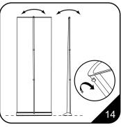
14. The unit can be leveled by adjusting the threaded plastic feet at the bottom of the base unit.
